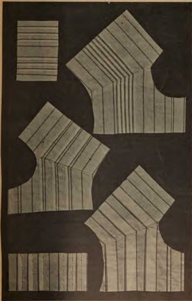
FIG. 70.—Several arrangements of stripes to form tucks or plaits, and match the stripes at shoulder seams.
